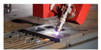
**HIGH DEF BEVEL PLASMA CUTTING** With a format cutting area of 10m x 2.5m as well as a fully rotational bevelling head, we are able to cut components up to 50mm thick.
