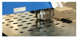
**CNC PUNCHING** Up to 2500mm x 1250mm x 6mm thick (stainless steel, mild steel, aluminium)
