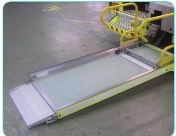
Deployed with the toe ramp down and ready to receive a stretcher or carry chair.
