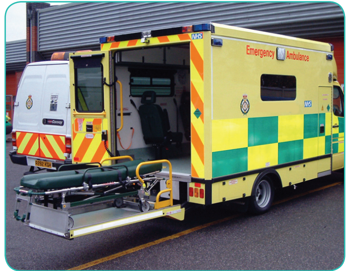
Lift being deployed showing the toe flap and the trolley stop in the 'up' position and safety handrails.
