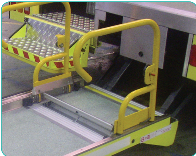
'StepSafe' foot protection fitted as standard to allow the use of wanderlead controls.
