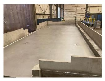
The table is 4.5m long by 2m wide and made of 40mm thick High Grade Duplex (Stainless) Steel has a 30-year operation life and must provide a flat surface with a fall of 1:90 to drain liquors to one end of the table.
