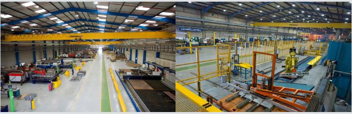
MTL Cutting Bay at our Rotherham based manufacturing plant housing a 20m x 3m capacity waterjet machine, 7 laser machines and 2 plasma cutters.
