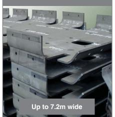
With 23 CNC press brakes available in-house and the capability to press metal sheets up to 7.2m wide, we can handle parts of the most intricate shapes and sizes from small sheet metal brackets to large pressed components.
