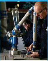
To ensure we consistently produce high-quality components and assemblies, we continuously invest in the latest state-of-the-art inspection equipment, including large format CMM machines with capability of up to 1200 x 2200 x 1000 (mm).
