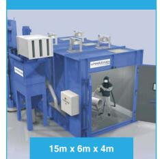
Our state-of-the-art air blast room facility is ideal for large scale components as we have the capability to blast material up to 15m long, 6m wide and 4m high.
