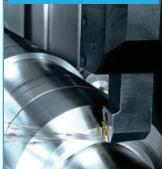
Our CNC lathes with driven tooling and sub-spindle options enable us to turn components up to 3.8m length, 950mm diameter.
