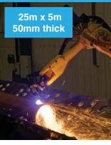
Our high definition plasma cutting technology with bevel capability has a large format cutting area of 25m x 5m with twin cutting head technology, allowing cutting of components up to 50mm thick.
