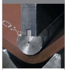
We specialise in cold forming and rolling steel and aluminium plates, a process involving zero heat input and does not affect the mechanical properties of the bent/ folded components.
