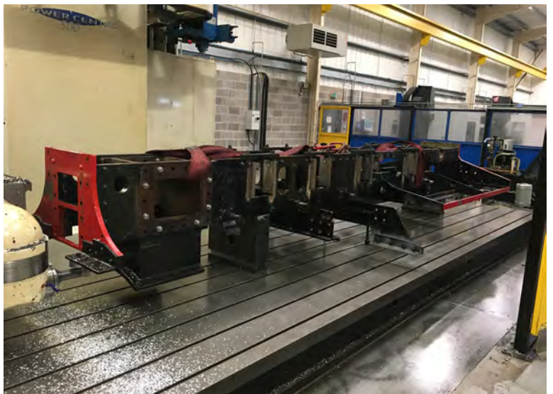
The steam train chassis was machined using our Asquith Butler Large Machining Centre
