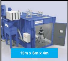
Our state-of-the-art air blast room facility is ideal for large scale components as we have the capability to blast material up to 15m long, 6m wide and 4m high.
