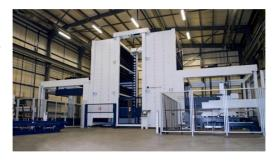
The equipment was made up of two 5kW TRUMPF TruLaser 5040 fiber laser cutting machines (4m by 2m format) with BrightLine fiber technology and SortMaster part sorting automation.
